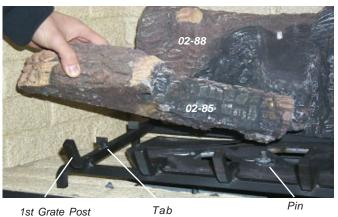
5) Line up the two holes on the underside of Log <u>02-86</u> with the 2 pins on the right side of the burner and position into place.
